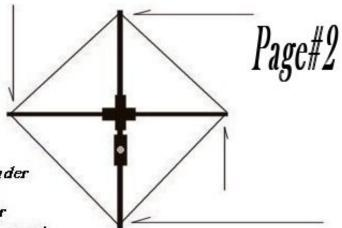
Drill holes in each spreader 14.5 inches from center of 1/2 PVC-X fitting, for driven Element. Measurement on Reflector is 15 from center out each spreader.
