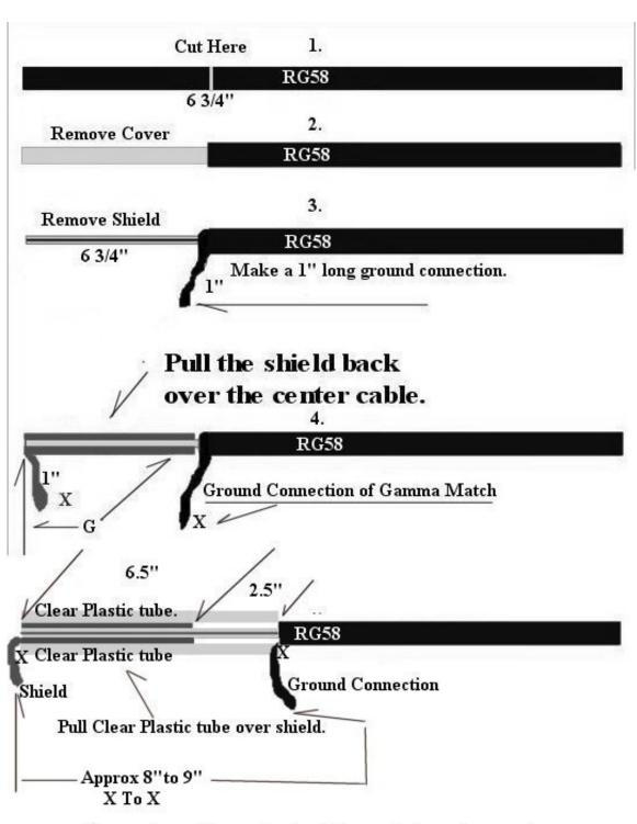
Be sure to weather seal ends of Gamma tube and connections with RTV or liquit electrical tape.
