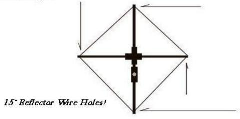
Remember! Measure from the center of the Cross Fitting out to find measurement!
